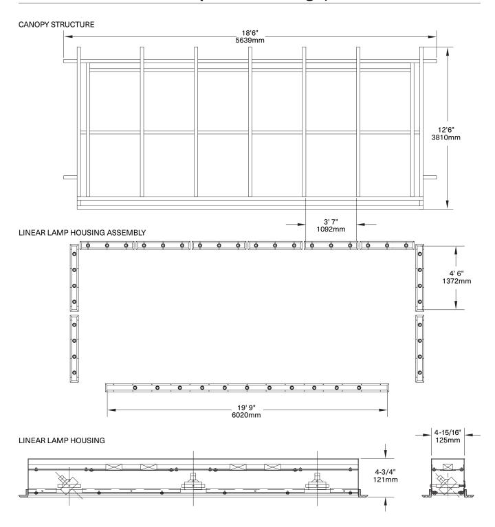
Custom fabricated aluminum linear channel incorporated with MR16 adjustable lamps with integrated electronic transformers. Fixtures designed to fit within the confines of the renovated hotel entrance canopy structure with matching powder coated finish.
